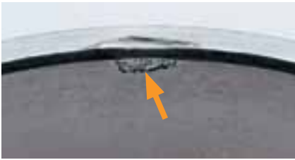
Cup-face denting: Indentations from hardened driver.
