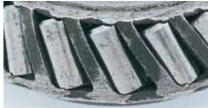
Rollers binding and skewing: Cage ring compressed during installation or interference during service.
