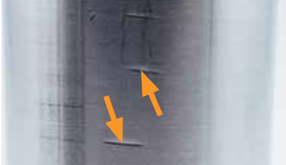
Roller nicking/denting: Rough handling or installation damage.
