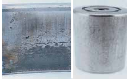
Micro-spalling due to thin lubricant film from high loads/low RPM or elevated temperatures.
