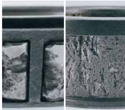
Rapid and deep spalling caused by unusually high stresses. Full race width fatigue spalling is caused by heavy loads creating a thin lubricant film and elevated temperatures.
