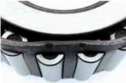
Cage Deformation: Improperly installed or dropped bearing.
