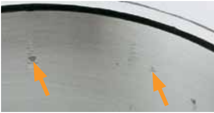
Roller spaced nicking: Raised metal on races from contact with roller edges.
